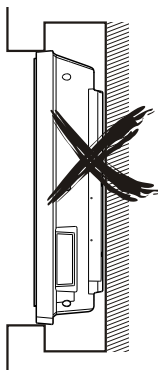
Air circulation is blocked
